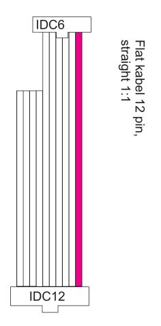
This is top view, the holes in the IDC/SPEEDY connectors are at the bottom (not visible in this view)
