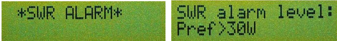
Fig. 10: SWR ALARM menu and adjustment
