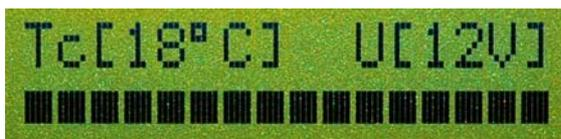
Fig. 7: *View type 3 (temperature, measured power supply voltage and adjusted output power; bar-graph in bottom line)*
