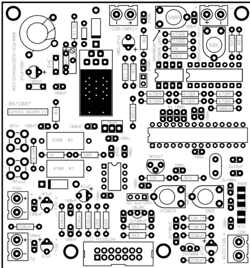
Fig. 2: Amplifier Control Board v20
