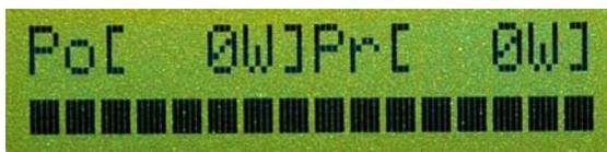
Fig. 6: *View type 2 (measured output power, measured reflected power and adjusted output power; bar-graph in bottom line)*
