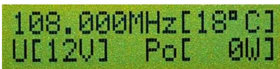
Fig. 8: *View type 4 (Frequency, temperature, voltage and measured output power)*
