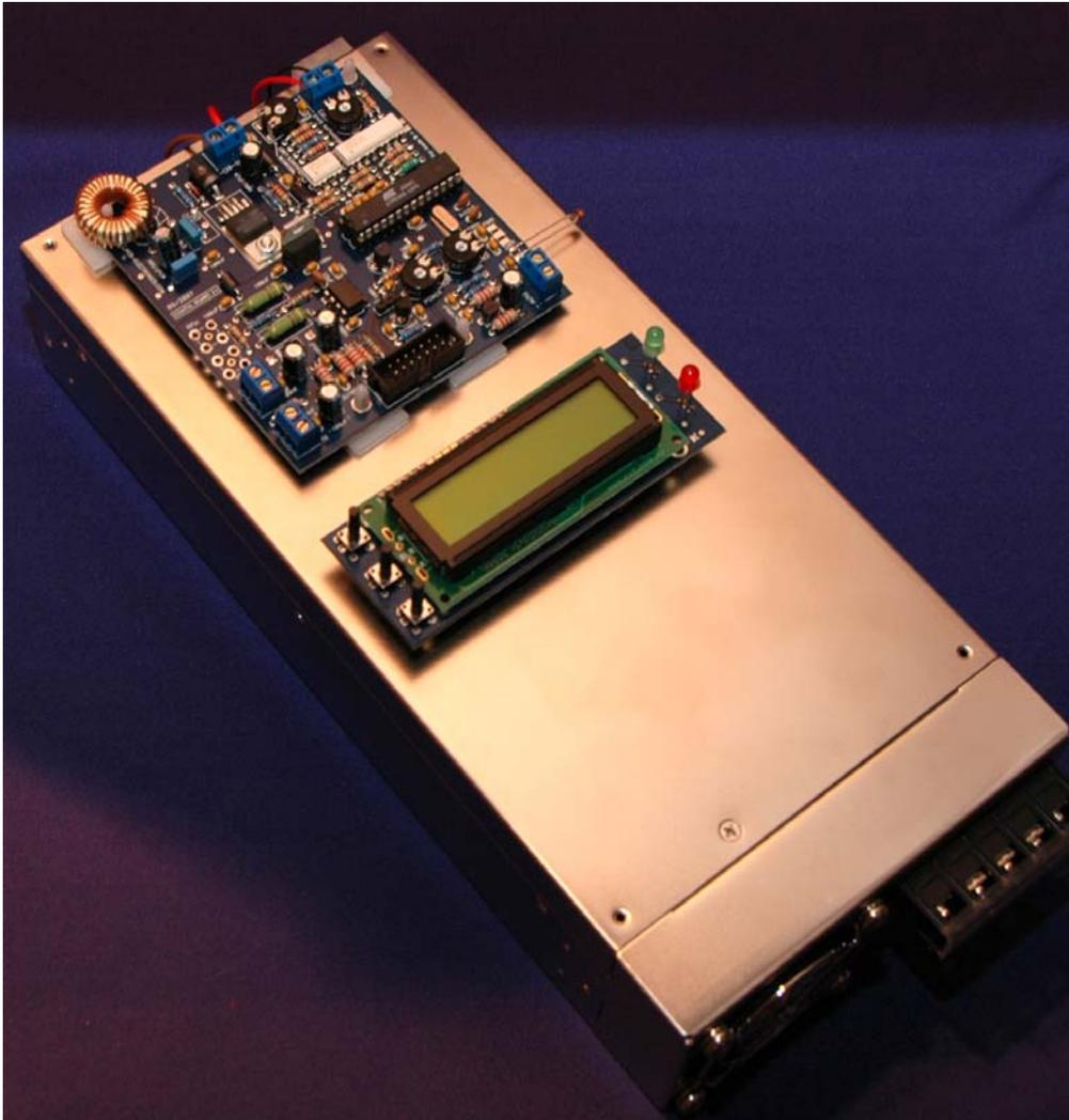
*Fig.1: Universal Amplifier Control Board 2.0*
