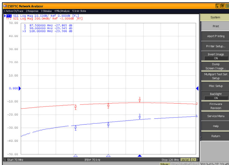
Input Return Loss and Insertion Loss
