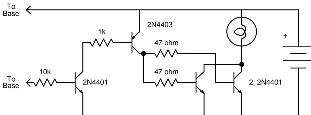
MAGIC LAMP: A single 2N4401 driving the lamp will work with a slight reduction in brightness.
