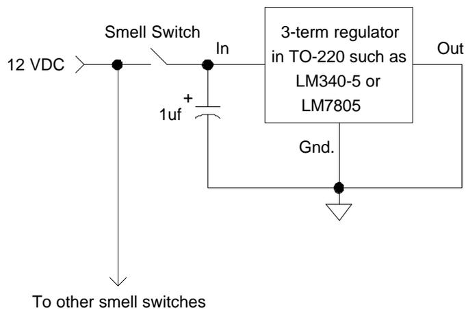
Smell Generator Schematic: The capacitor is optional since the regulators aren't likely to oscillate in current mode and even less likely in thermal limit mode. Add them if radio interference is encountered.
