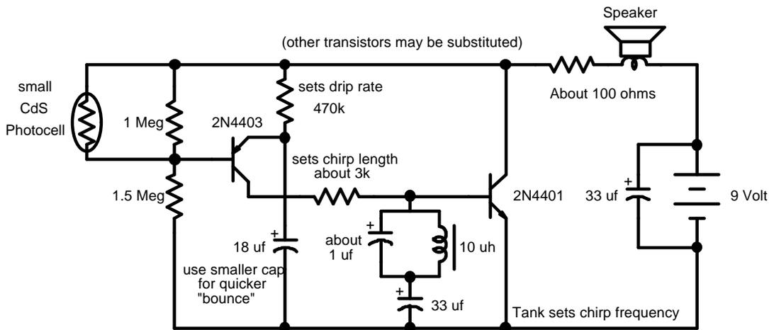
THE DRIPPER: Don't hesitate to vary any values. A little experimenting will yeild a superior drip sound.
