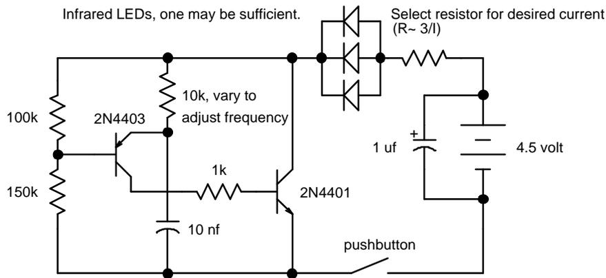
REMOTE CONTROL JAMMER: Increase the resistor in series with the LEDs to prolong life. A fairly weak signal will usually do the trick.
