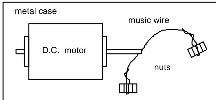
Figure 1: Motorized "really bad sound" generator.
