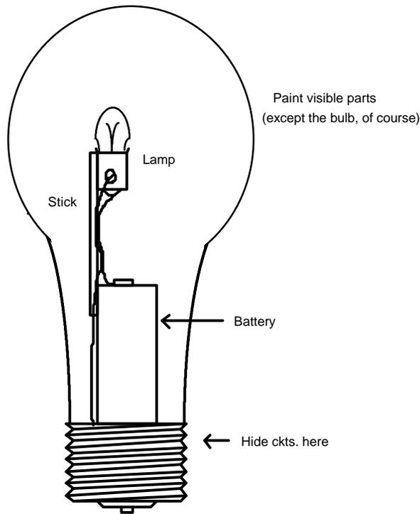
Several factors should be considered when selecting a battery and lamp combination. First, the weight should be kept low if the victim will hold the bulb. Second, the lamp should be as bright as practical and should emit light in an omnidirectional pattern. Try those "super Krypton" flashlight replacement bulbs and two AAA cells or one AA cell.
